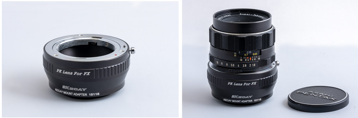
FIGURE 06: This is a typical lens adapter; in this case it adapts Pentax screw-mount lenses to a Fuji X camera. I used it to adapt this Pentax lens from the early '70s to my Fuji X-T3. There's no autofocus and you have to shoot in Manual mode, but the camera's light meter works fine.
